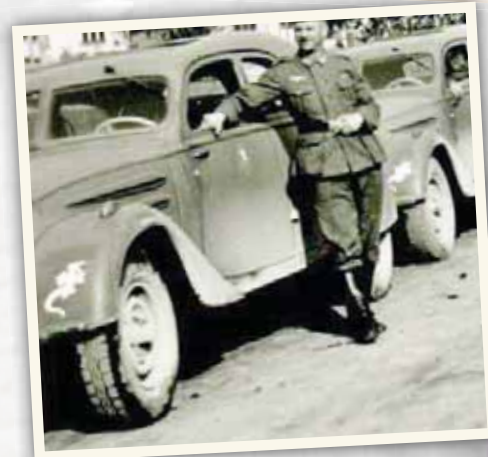
These 402s seem to have larger Michelin tyres and an increased ground clearance.
