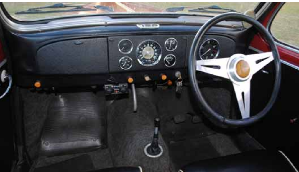
The short stubby floor mounted gear lever, the black interior colour and the bucket seats with white piping are a real giveaway that this is a modified interior.
