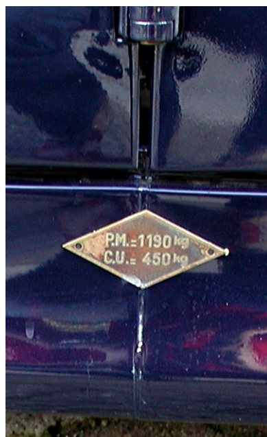
Sander's 203 has a brass load plate under the B pillar.
