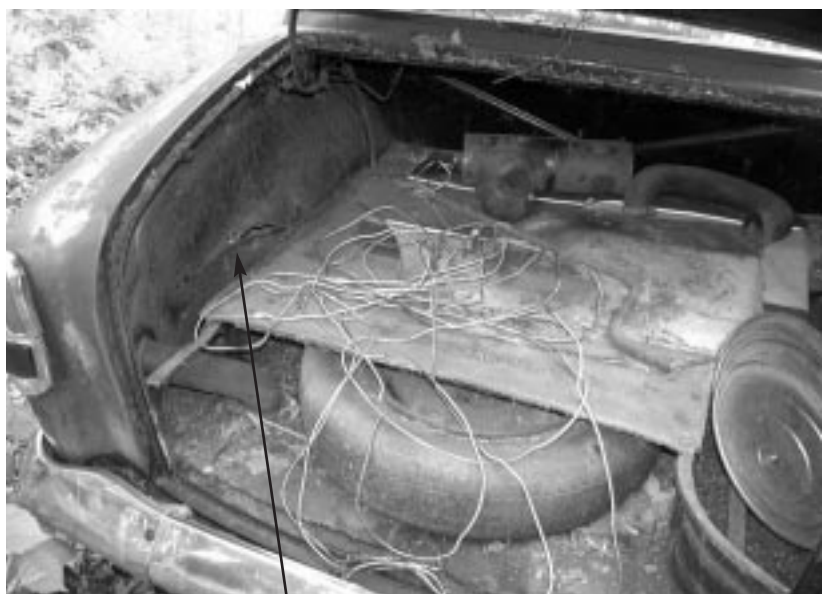
403 boot showing the typical rust to check for in the fold in the inner guard. Picture from a series of pictures a 403 "for sale" on the internet auctions. US$600 asking. Rust free they said!
