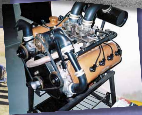
Jim Hawker built a V8 for his 403 from two 203 engines.
