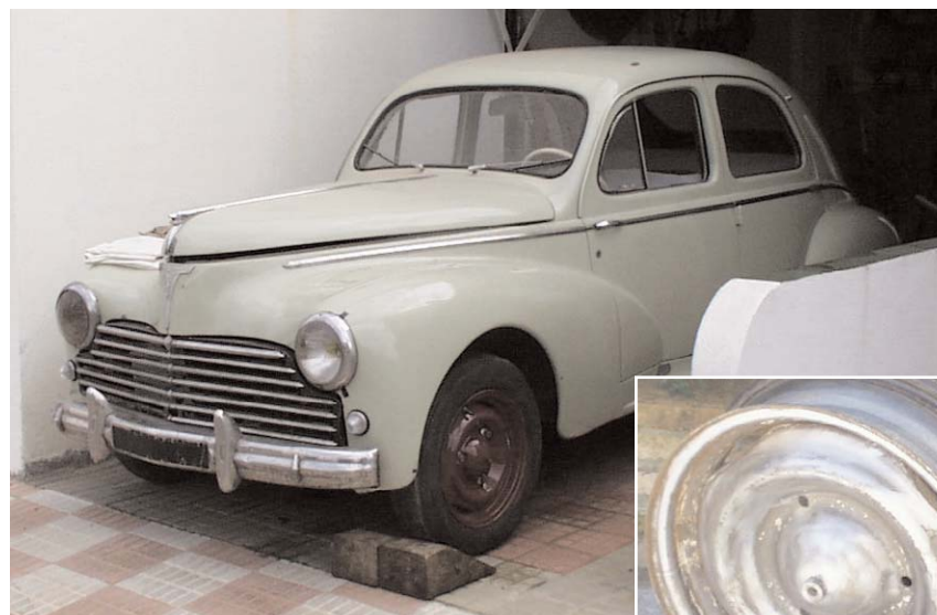
203 owned by Juanma Herrera in Spain. Restoration nearly finished. Note the 203 wheels for bolt on hubcaps.
