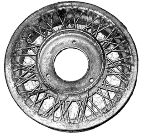
These mock wire wheels are much sought after in France. They were made by Robergel. Note how the spokes were combined with the 203 three stud hub.
