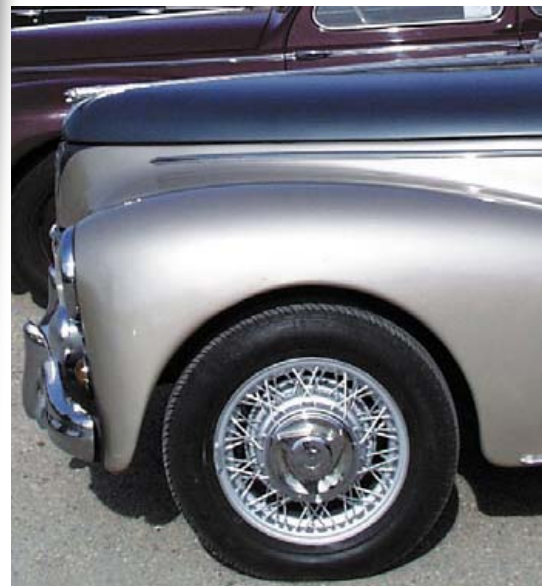
These mock wire wheels are much sought after in France. They were made by Robergel. Note how the spokes were combined with the 203 three stud hub.
