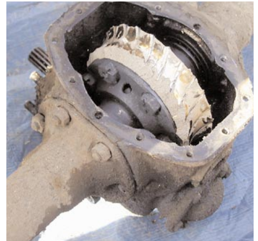
The bronze worm wheel in the differential failed in Addis Abeba.
