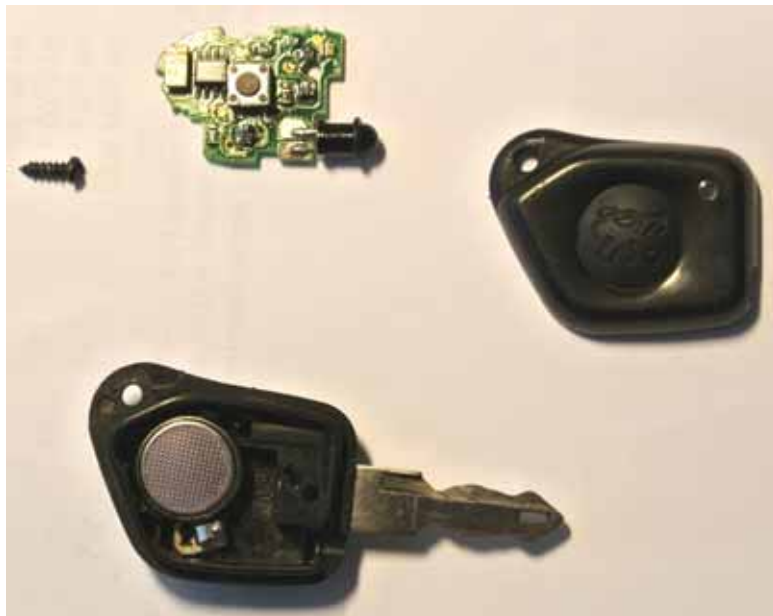
Circuit board with new pushbutton, cleaned up key shell with new batteries, ready to reassemble.
