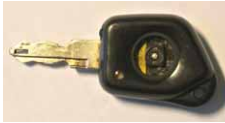
Non-functional 306 key with plastic cover gone and switch broken.
