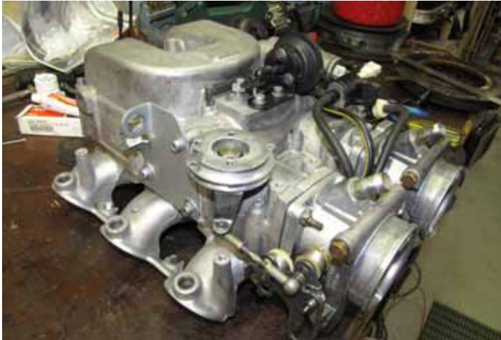
The inlet manifold is a large complex piece of hardware. Solenoids control two internal sets of butterfly valves to alter inlet tracts and volumes. Throttle control is by two Weber 55mm throttle bodies and idle control is by a Bosch air control valve. The acoustic physics in the design of this manifold require the inlets to the air filter be re-joined within a few hundred mm of the manifold before the air filter.
