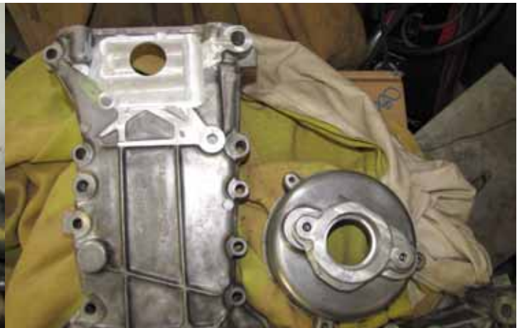
HT Distributor and timing cover: Much time spent on my milling machine here to allow the high tension distributor to sit on the driver side of the timing cover. It had to be in the right spot, it had to have an oil seal and the rotor had to be timed.
