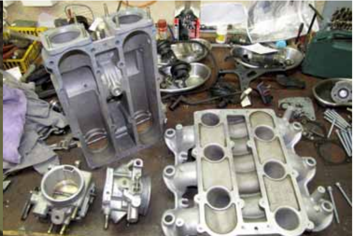
Here are the four key components of the inlet manifold, the two Webber throttle bodies, and the upper and lower castings of the manifold. The centre void is used as a vacuum reservoir for the control valves. Note some of the internal control butterflies are visible.
