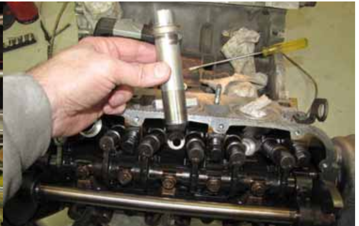
Spark Plug tubes: Perhaps in a nod to older Peugeot engines ('older' as correctly defined by Mark Besley) the spark plugs are down tubes that sit inside the rocker cover. I had to remove and reseal these as all of them kept filling with oil.
