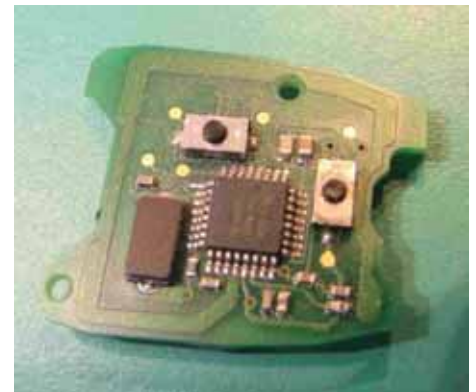
Circuit Board Removed from Old Key – Note the Lock and Unlock Buttons
