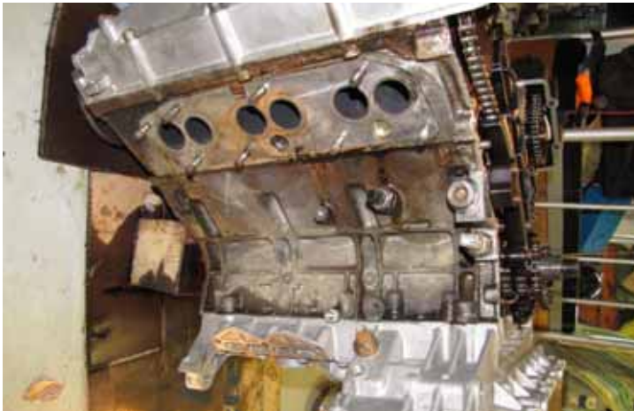
Motor side view 6 ports and new sump: Count the exhaust ports! I was not expecting this although M116s use a similar design. Note the Volvo/604 style sump.
