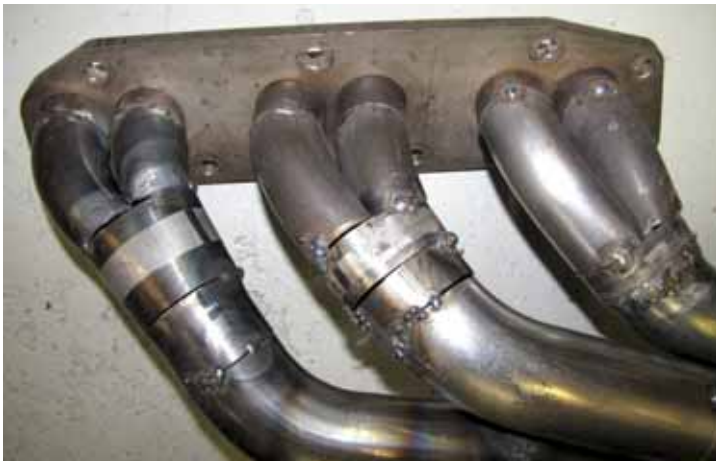
Exhaust headers: The Frankenstein of exhaust headers. Two 30mm ports are merged into a single 42mm pipe close to the manifold. These lead to a large collector and 2 inch secondaries.
