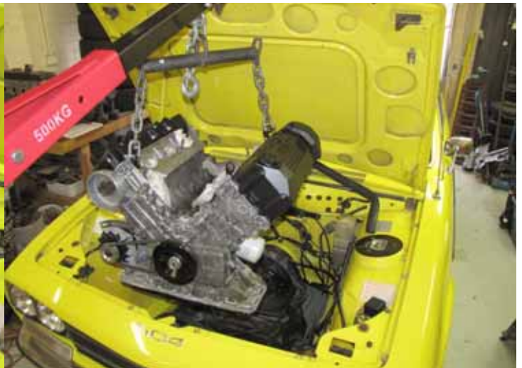
Evenfire 24V in: The Citroen motor fitted with a Volvo sump being lowered into a 504 Peugeot. I really liked doing this bit.
