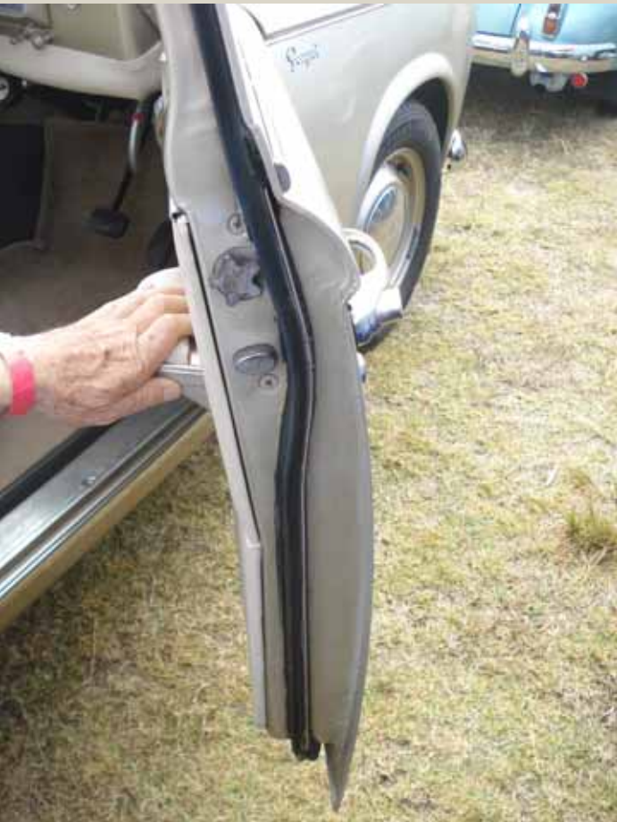
The Wilkinson method for fitting 403 door rubbers.
