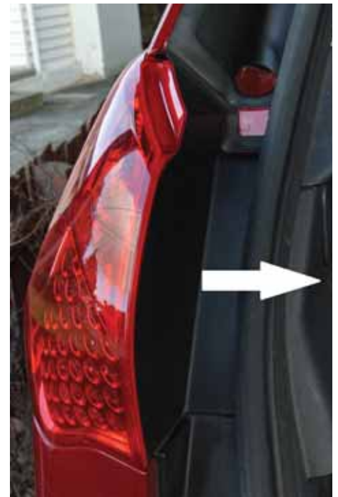
Plastic cover needs to be removed in the direction of the arrow.
