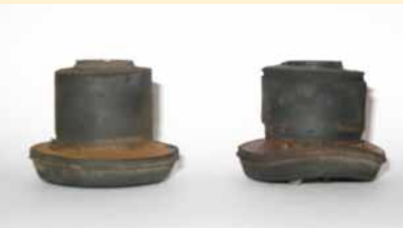
Left hand bush was okay but one on right has obvious wear. Yes, I accidentally bent the steel washer.
