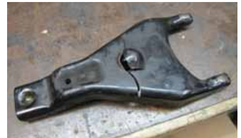
A cracked 505 clutch fork, more common than it should be.
