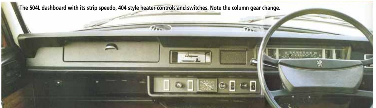
The 504L dashboard with its strip speedo, 404 style heater controls and switches. Note the column gear change.
